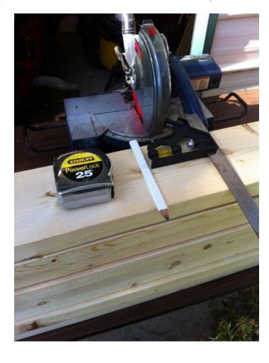
1. If you are using a mitre saw a heavy line is not always needed. Arrows can help show the exact point you were marking.
