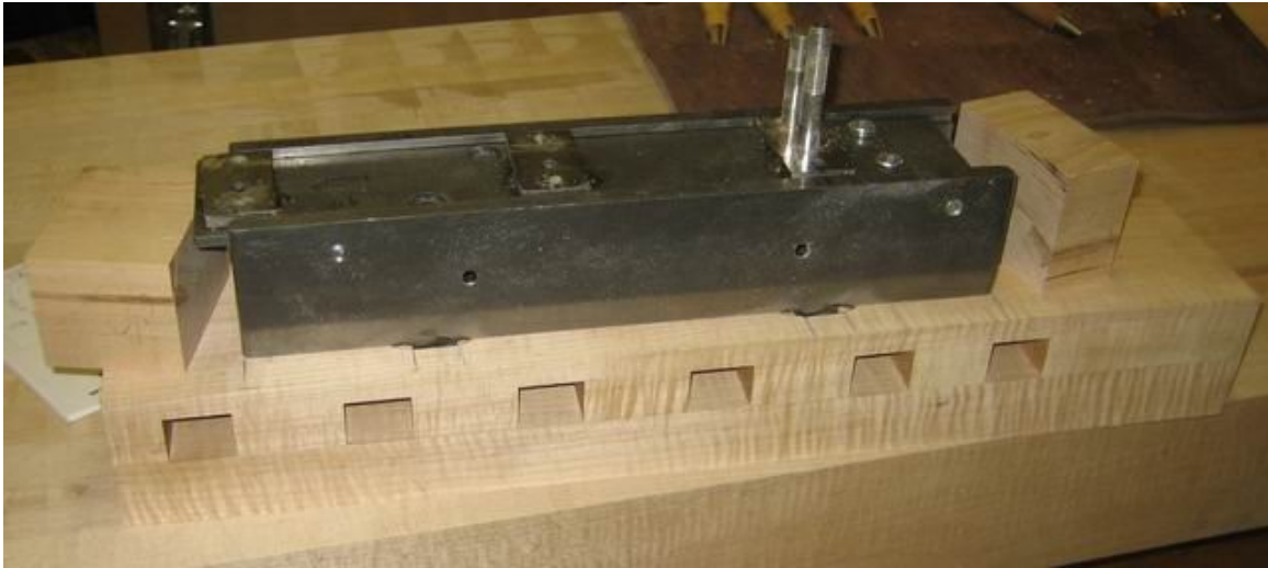
Tail vice assembly. Spacer blocks are glued to doghole strip. Then cover plate is glued on top of spacer blocks and is screwed to the welded assembly
