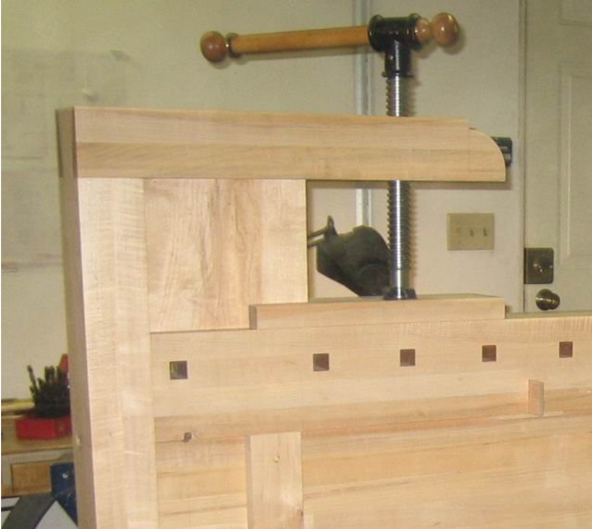
Underside of shoulder vice showing vice jaw and arm riding under the spacer block. Spacer block is allowed to expand/contract to the right side of the picture. Splines on left side of spacer block are glued.
