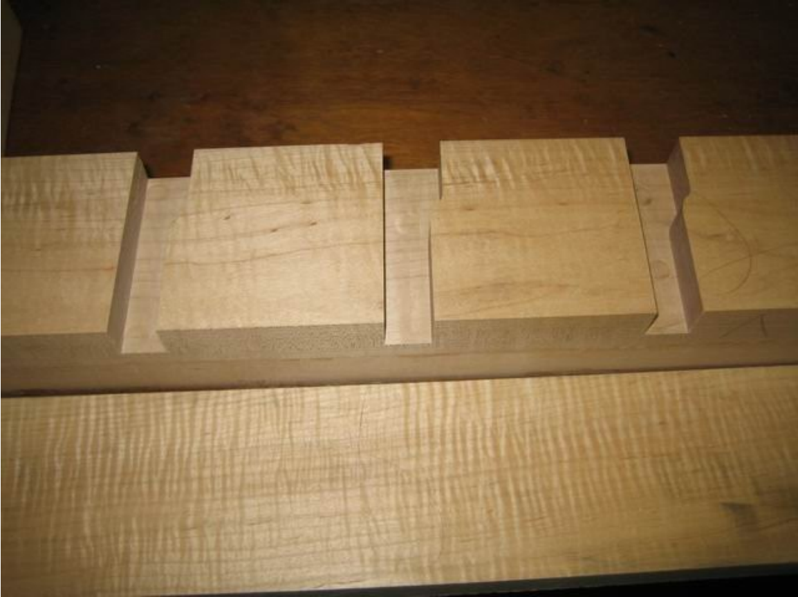
View of dogholes before cover strip glued on
