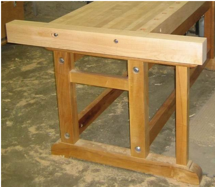
Shoulder vice end end cap showing bed bolt locations.
