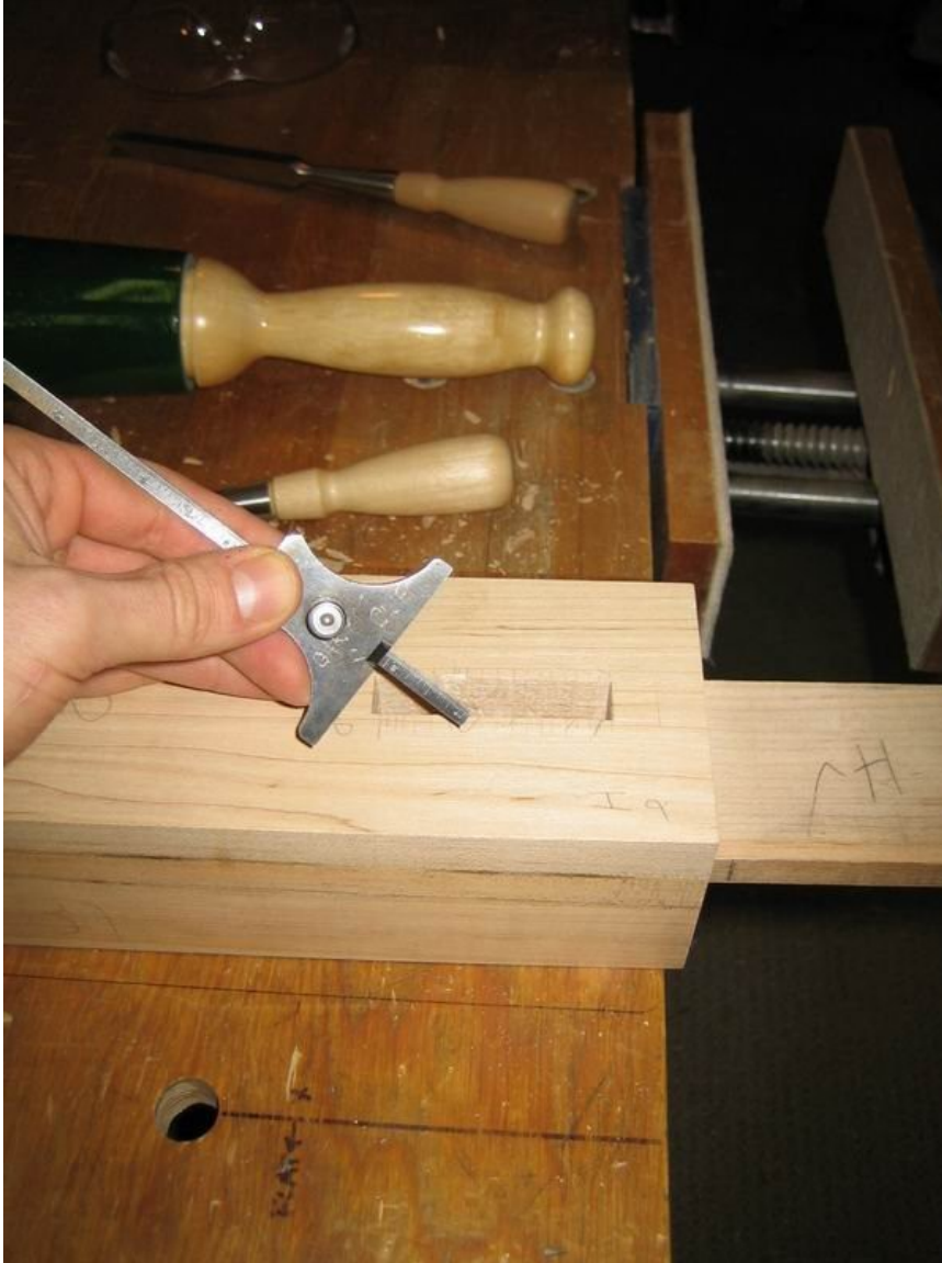
Chopping mortises checking to see if ends and sides are square
