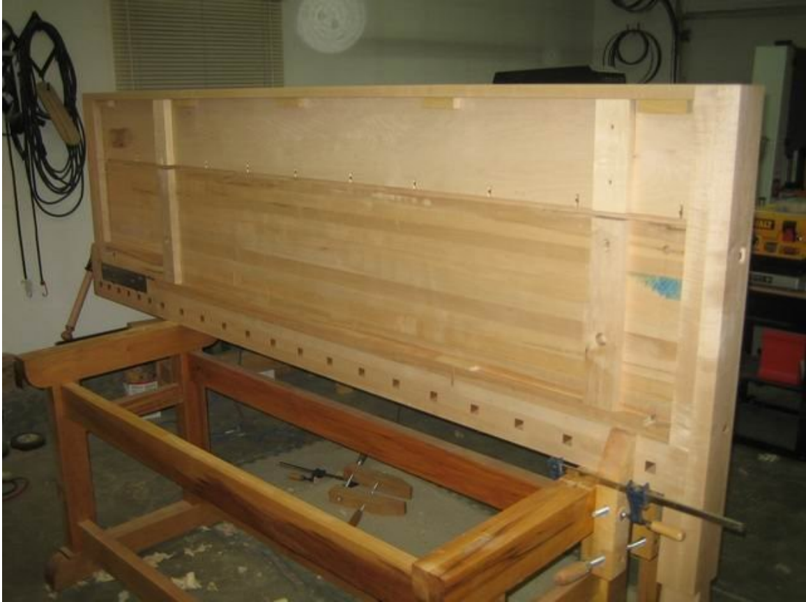
Underside of bench showing tool tray bottom, glue blocks, slotted screw holes, and spacer blocks
