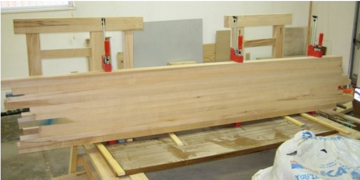
Benchtop boards laid out for best grain direction
