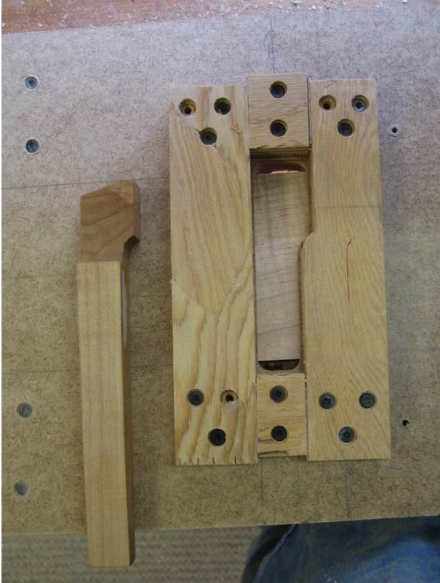
Benchdog and benchdog router template – top view
