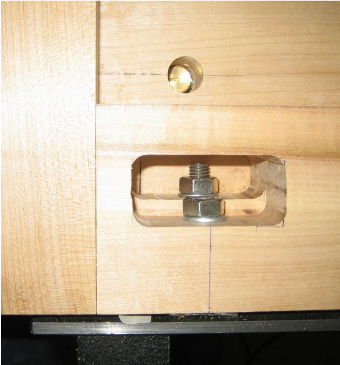
Underside view of mounting bolts (mounting plate visible at bottom of picture). The brass nut visible at the top is one of the bed bolts holding the end cap in place.
