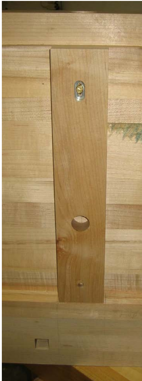
View of underside filler strip
