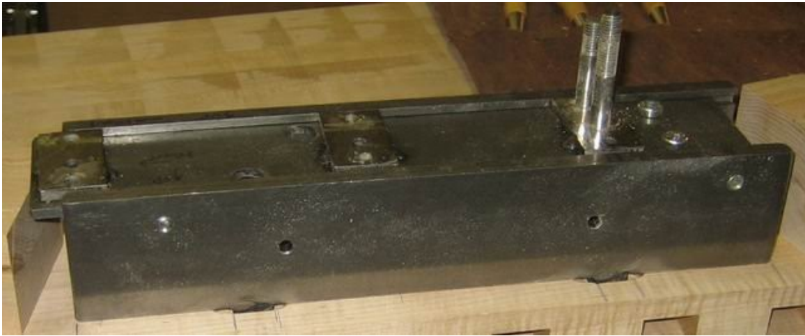
Small welded tail vice hardware view from backside (note I modified one of the bolts to be shorter than the other bolt). Handle end of the vice is to the right and upper side of vice is in foreground of picture.
