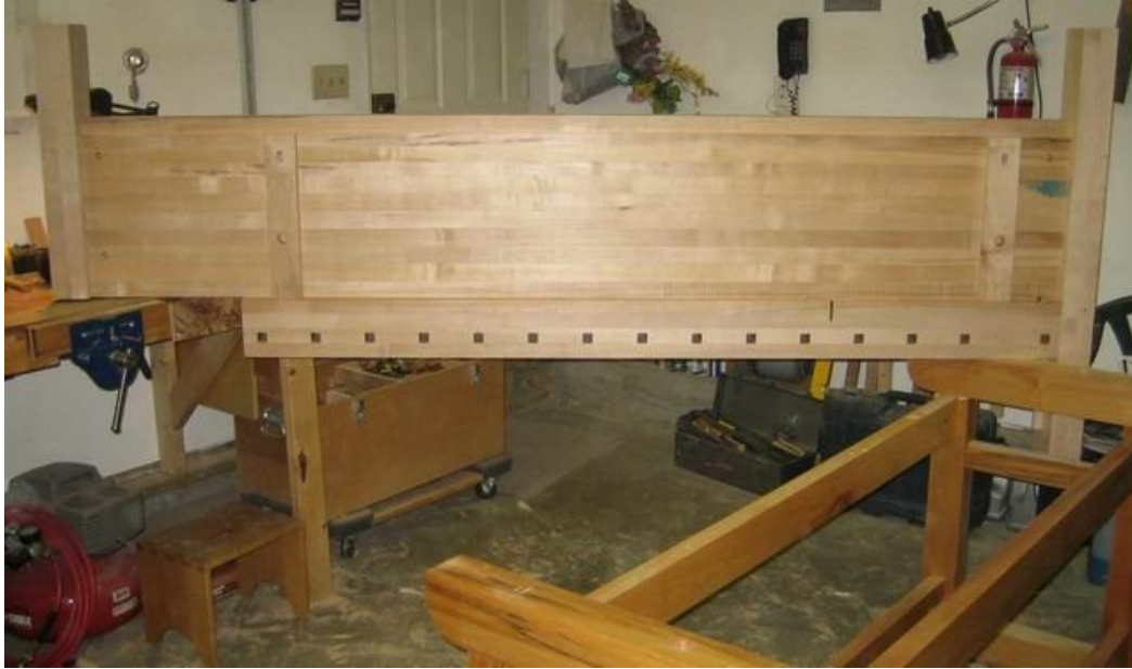
End caps in place. Benchtop is getting very heavy. I had to turn the benchtop 180°. With only one person, it was a difficult task.
