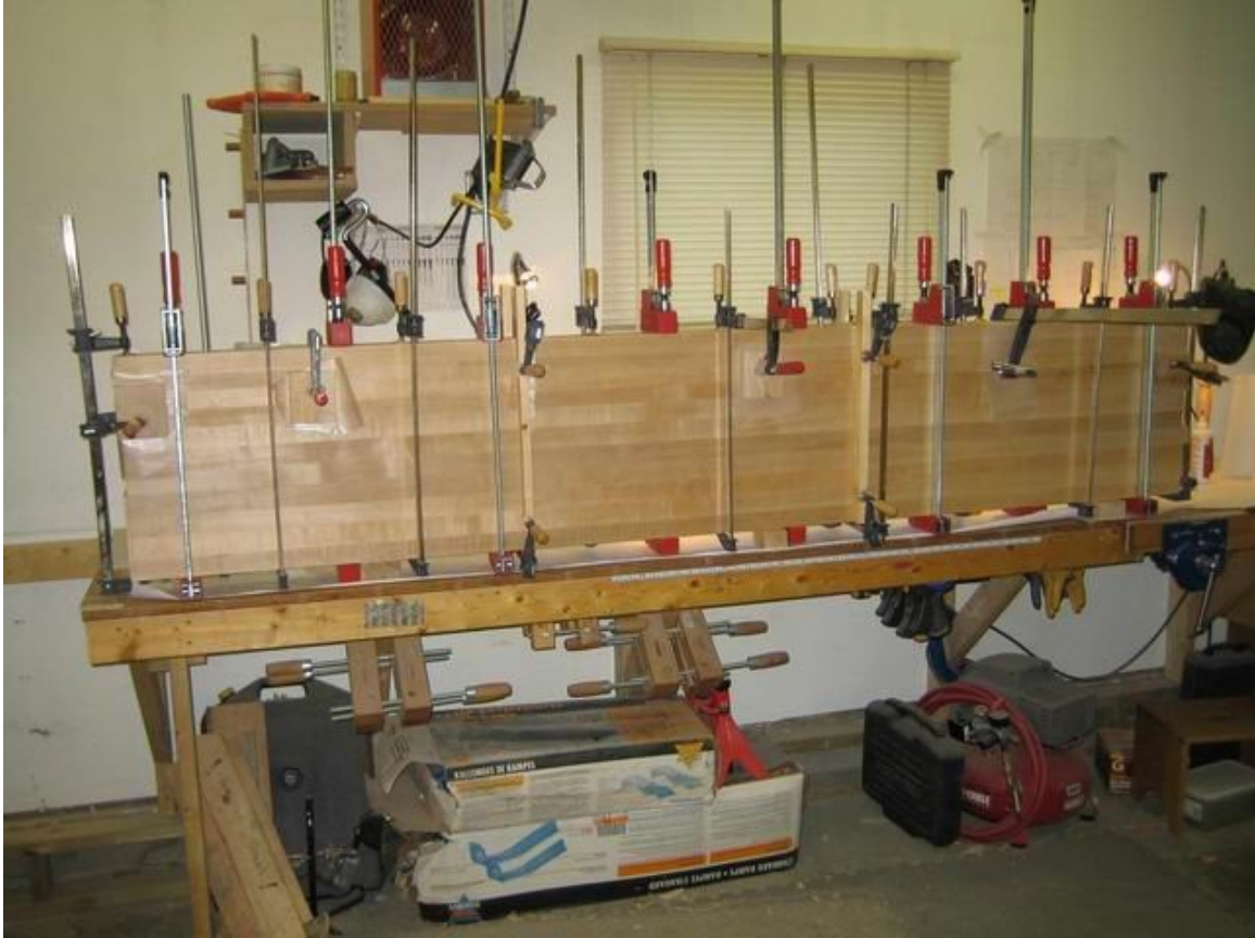
3" thick part of benchtop being glued up
