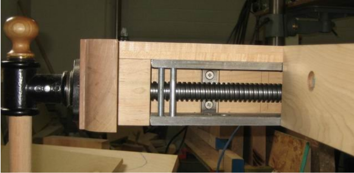
Backside view of tail vice assembly at maximum opening
