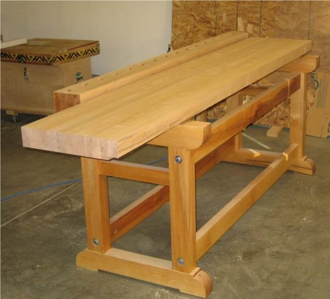
Benchtop before doghole strip glued in place (view from rear of bench) – doghole strip is 4” thick, remainder of benchtop is 3” thick.
