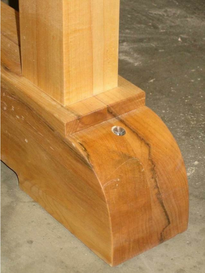
Completed foot showing leveller adjustment screw
