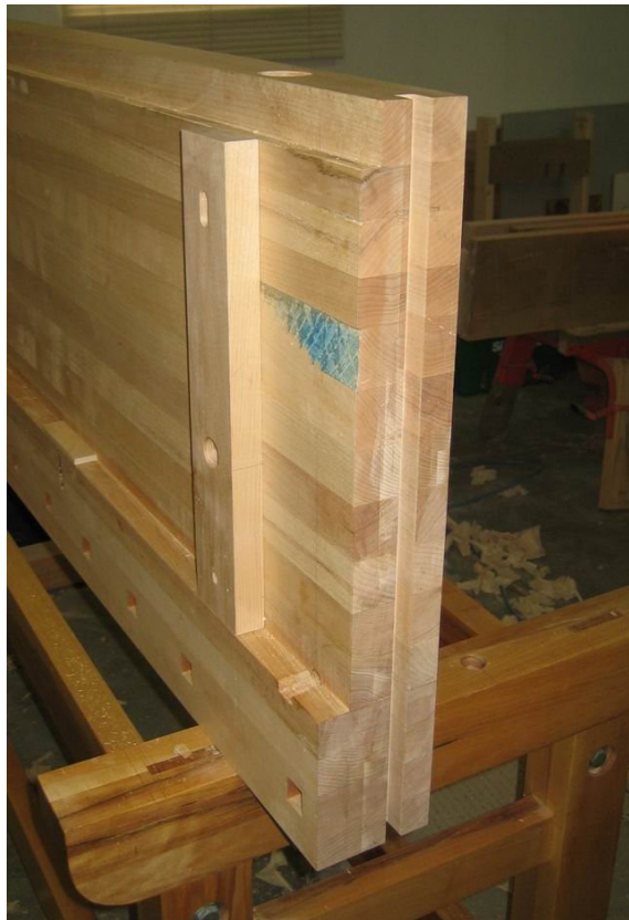
Spline groove formed in bench end
