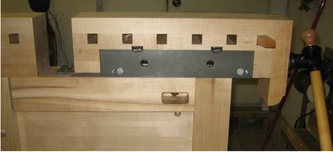
Underside of tail vice partially open position
