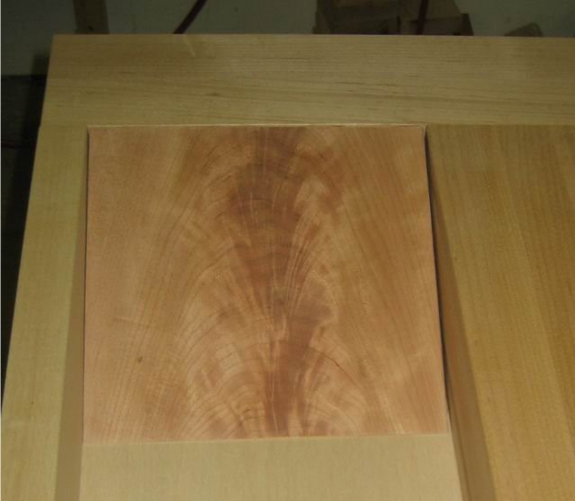
Finished tool tray ramp with cherry crotch veneer (approximately 1/8" gap allowed between plywood part of the tool tray ramp and the workbench to allow for expansion/contraction)
