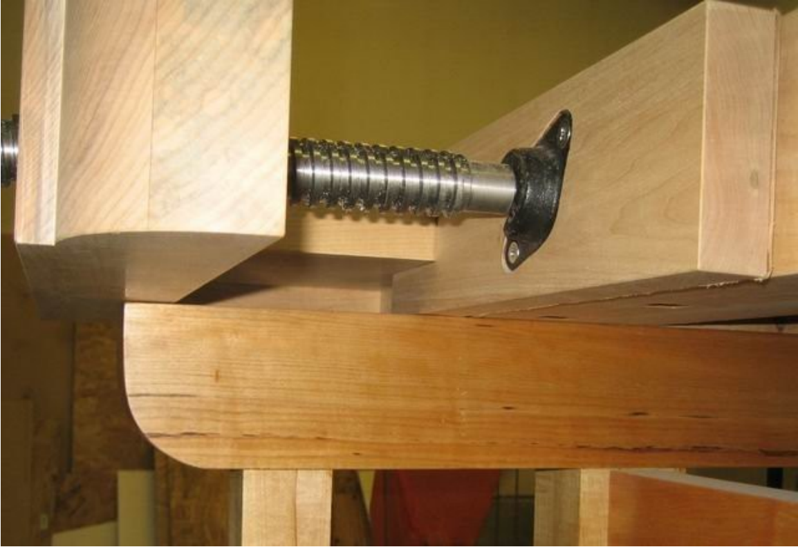
Side view of shoulder vice showing arm riding on top of base
