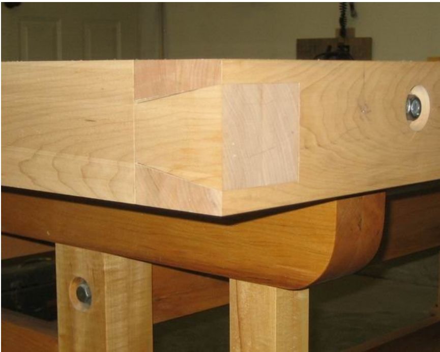
Assembled shoulder vice dovetail before glue up
