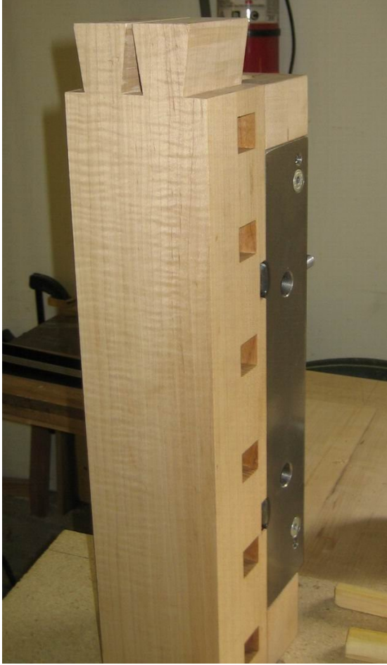
Dovetails cut for the tail vice assembly end cap
