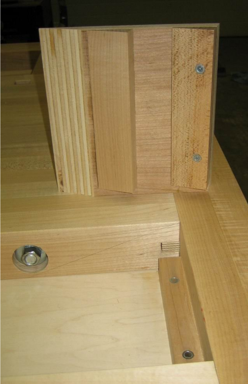
Tool tray ramp magnets (square block is glued to end cap)
