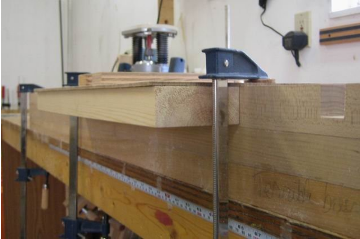
Benchdog template clamped in place – underside view showing one of the 2x4 guides
