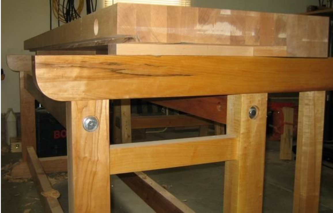
Doghole strip glue to main body of bench place. Filler strips under the 3" thick section of the bench are in place. Hole for shoulder vice threaded rod is visible at back of benchtop.
