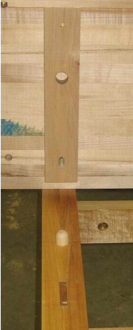
Underside of bench showing filler strip and bullet dowel
