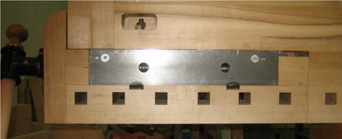
Underside of tail vice closed position. Note that the jaws close very tightly to each other. By ensuring that the ends of the tail vice and the dog hole strip were perfectly square before glue up and assembly of the vice the jaws fit perfectly and I did not have to make any corrections.
