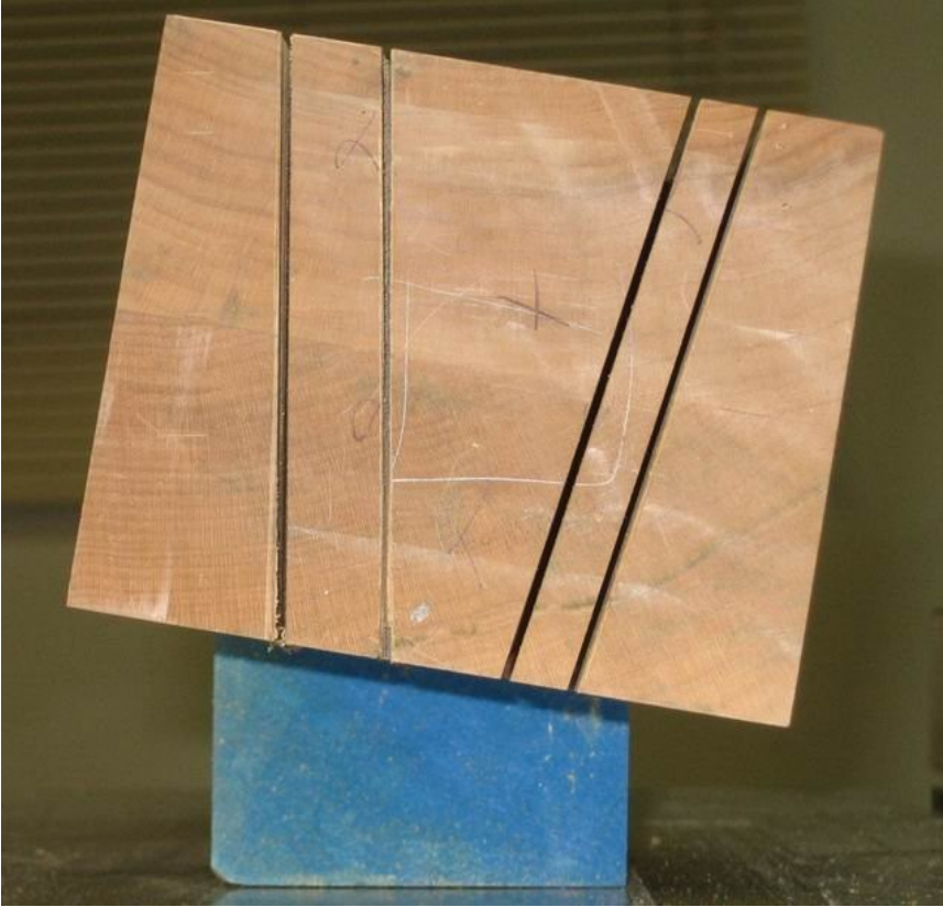
Cutting the shoulder vice pin board on the bandsaw using an angled guide. Inside cuts were practice cuts. Outside cuts were cut very close to the line on bandsaw, then were cleaned up with a #60 1/2 rabbet plane.
