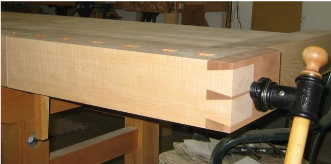
Finished tail vice (note undersized diameter handle) – March 13, 2006
